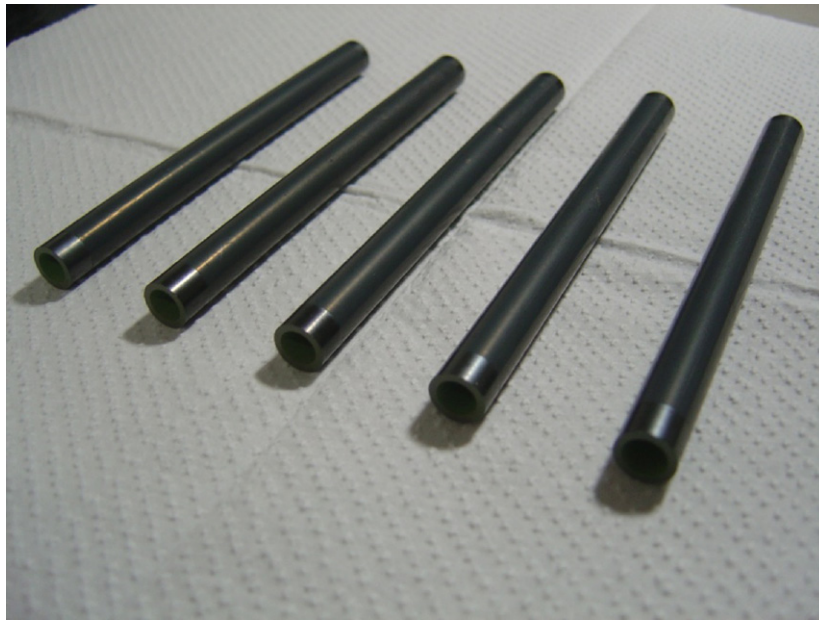
Fig. 2. Photographs of the prepared micro tubular cell.
